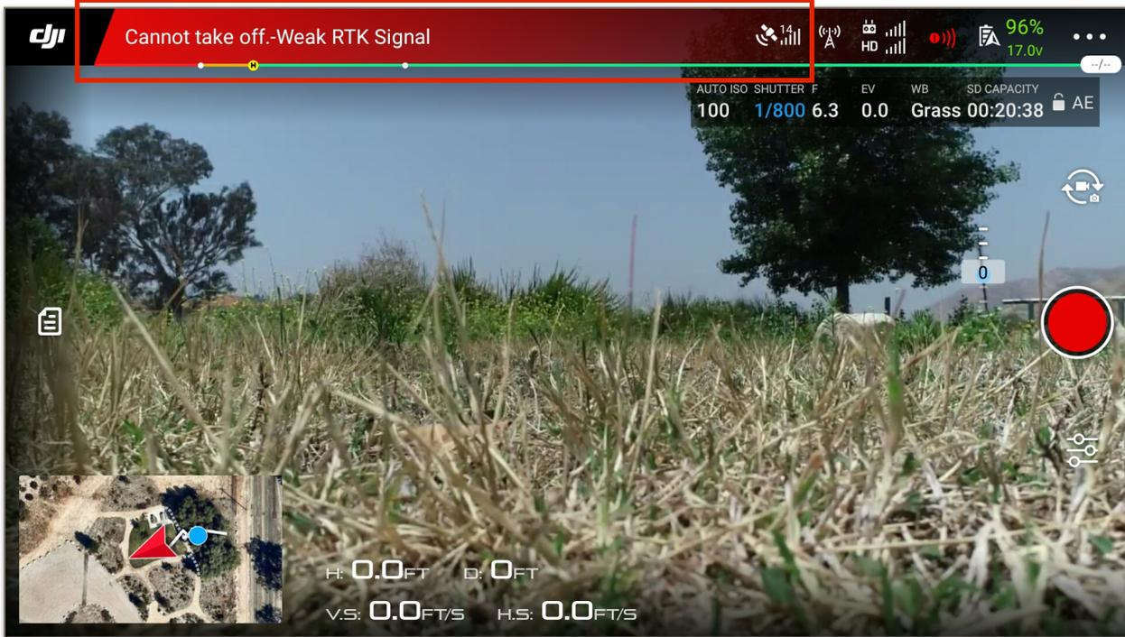
Once the GPS/GNSS signal is sufficient for operation, the error would automatically disappear, the aircraft position status would be changed to “FIX” on the status bar and “RTK Settings” page:
